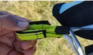
Insert the reserve into the container, taking care to fit the risers behind it, so that half of the reserve protrudes from the middle plane (rescue in a vertical position).
