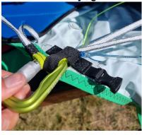
The accelerator is already in place, however, check that it is correctly routed and adjusted. You can shorten it or lengthen it on its connection to the pedal.
